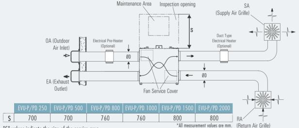
"S" values indicate the size of the service area. A service space of "C" must be left under the unit for fan service. Drain pipe must be installed.
