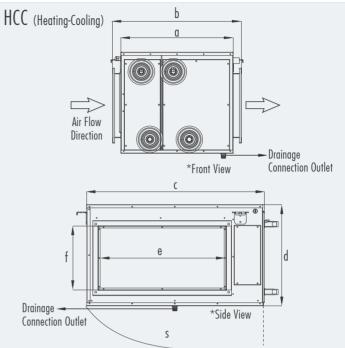
"S" value indicate the size of the service area. All connections are threaded connection.
