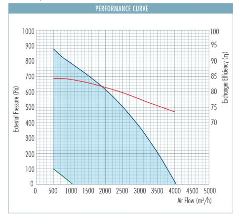
Note: Efficiency values are calculated according to EN 308 standard.
