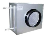
Duct type cooling and integrated heating coils are assembled in cabin as suitable to mount inside duct and have capacity. Coils consist of copper tubes and aluminum fins. Inlets and outlets of cabin are suitable for circular duct connections as in heat recovery ventilation units. Additionally, cooling coils have drain pan and extra insulation to prevent condensation of cabin.
