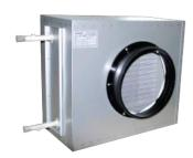
Duct type heating/cooling coils are assembled in cabin as suitable to mount inside duct and have standard capacity. Coils consist of copper tubes and aluminum fins. Inlets and outlets of cabin are suitable for circular duct connections as in heat recovery ventilation units. Additionally, cooling coils have drain pan and extra insulation to prevent condensation of cabin. Both heating and cooling coils can be controlled seperately as on/off via unit automation system.
