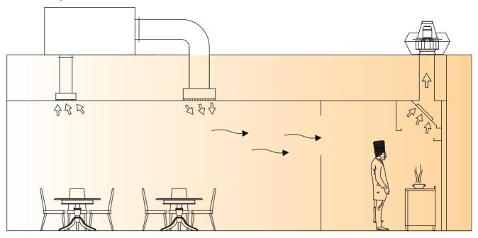
Ventilation system exhausts the conditioned air from the kitchen and neighbor areas. As the cooking appliances are not isolated from the kitchen, significant amount of air is exhausted to avoid cooking gas inflation to the kitchen and neighbor areas. For a medium kitchen, exhaust air temperature is 28 °C in summer and 24 °C in winter which results in significant energy losses.
