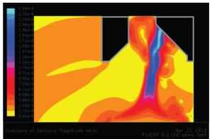
Engineering calculations are vital to simulate fluid characteristic. For complex models it is extremely hard to calculate the characteristics with analytic methods. Instead numerical methods are used to calculate heat transfer, pressure drop and flow velocity during design process to ensure alike behavior of the equipment in operational period. DES units are analyzed to calculate proper amount of fresh air and correct supply points in kitchen spaces with CFD-Computational Fluid Dynamic software.
